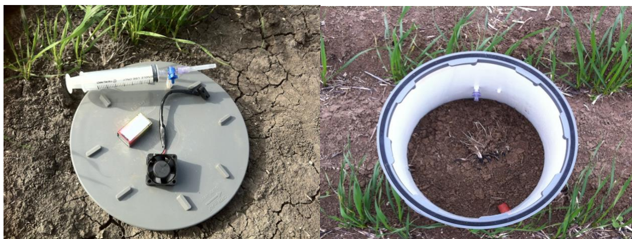
Figure 2: N 2 O sampling cylinder (right) with lid and syringe to extract samples from the cylinder (left)
