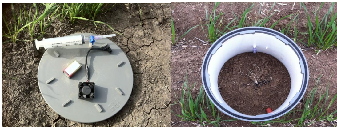
Figure 4 N 2 O sampling cylinder (right) with lid and syringe to extract samples from the cylinder (left)
