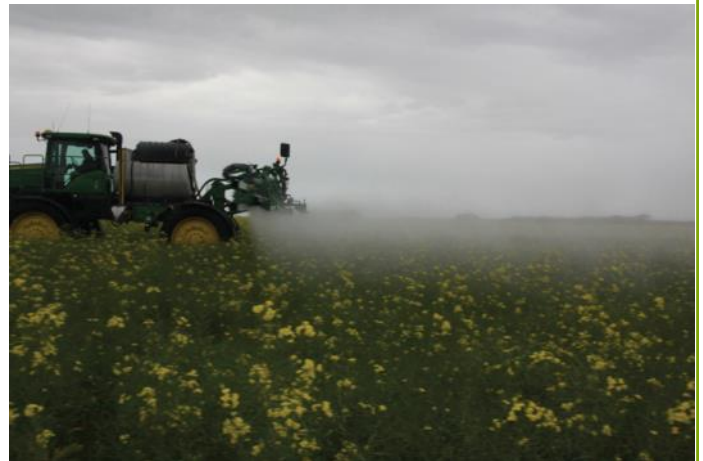
Operating at high spraying speeds with a fine spray quality can lead to excessive amounts of spray remaining in the air. PHOTO: Bill Campbell
