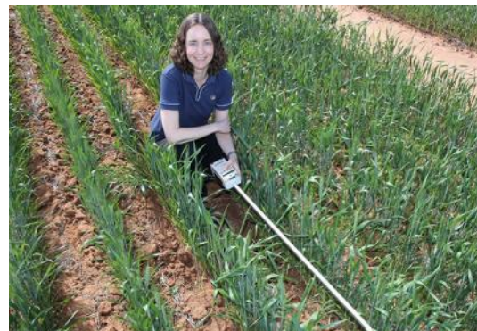
Dr Catherine Borger measuring light availability to the inter-row space in wheat with a Sunfleck Ceptometer (photo courtesy of Glen Riethmuller, DAFWA).
