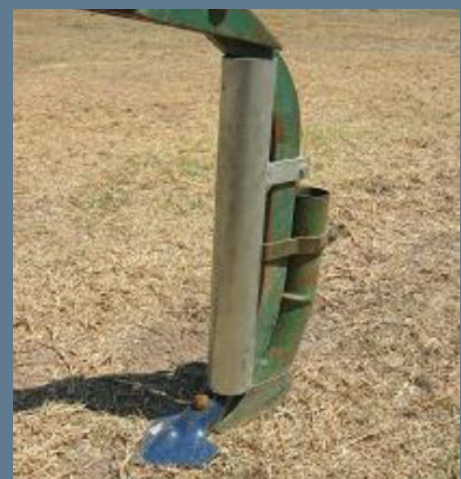
Left: The tyne vertical clearance, shown as 'H' is the distance from the ground to the first obstruction on the tyne shaft or mounting head. Photo: Jack Desbiolles
