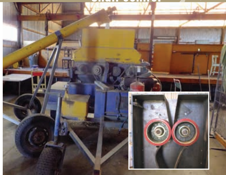
'Shmik' snail crusher grain roller, modified to increase throughput, and better manage small snails in canola. Photo: Michael Richards, Ag Excellence Alliance
