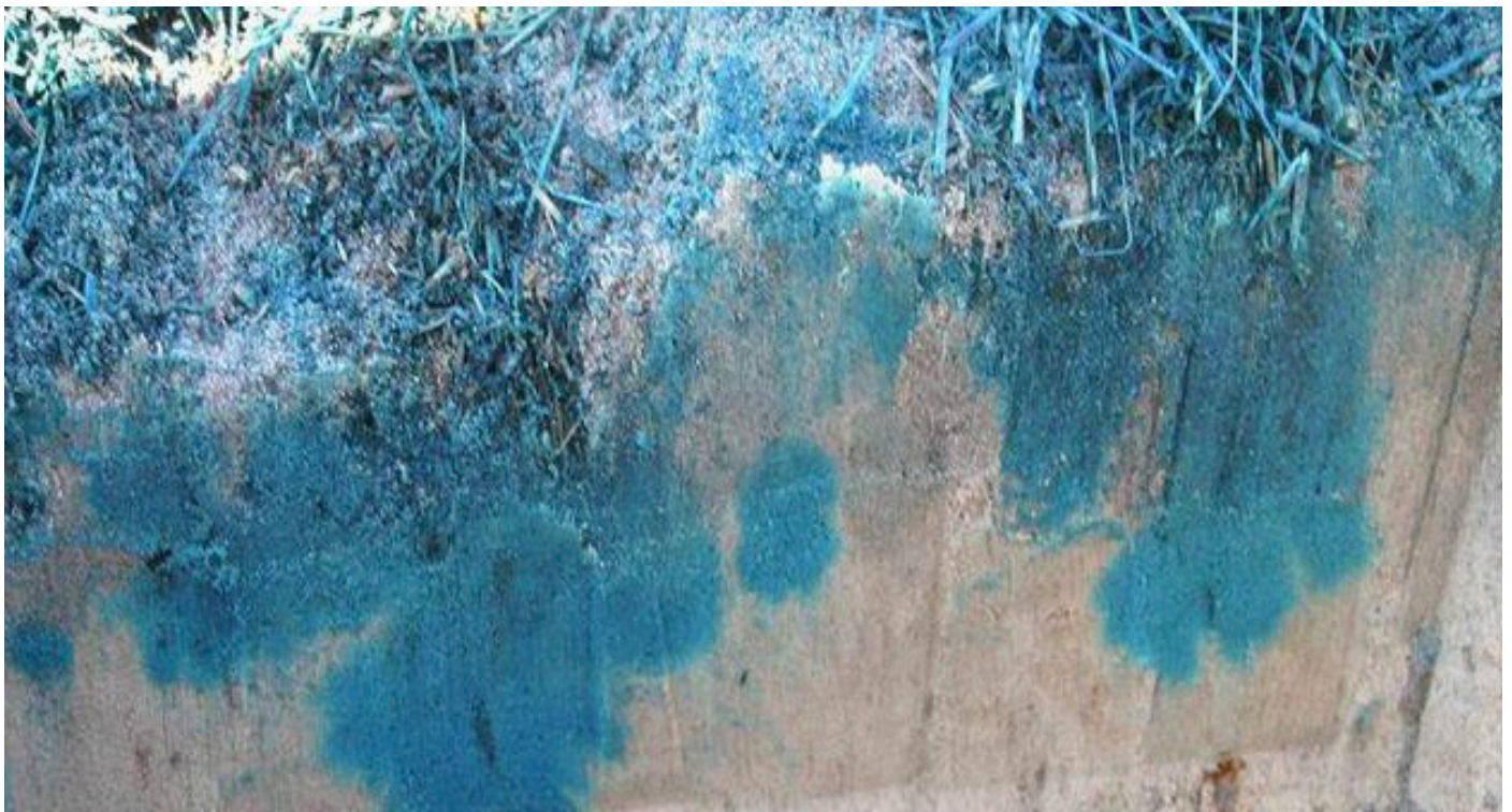
Figure 6. Non-wetting sand soil profile, using blue dye to illustrate the irregular infiltration of water down the profile (The Observer 2018).
