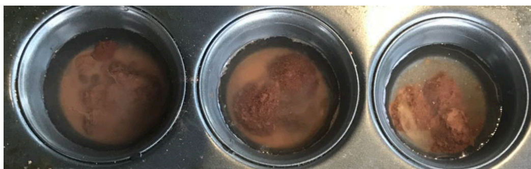
Figure 4. Example of simple dispersion test, with the sample to the left extremely dispersed and the sample to the right only moderately dispersed (Beth Sleep, 2021).
