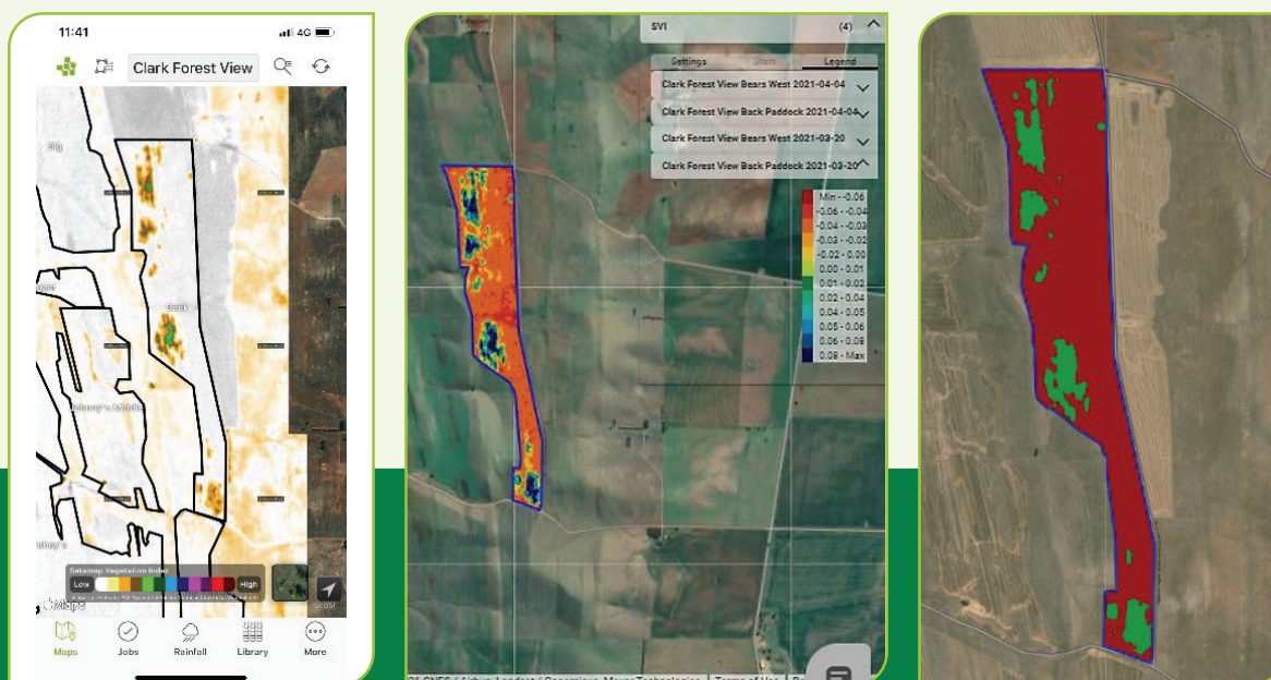
Fig 4 (left to right) – The Agworld SVI Image, the PCT AgCloud SVI Image, and the prescription made in PCT AgCloud. The green areas were sprayed and the red was left unsprayed.
