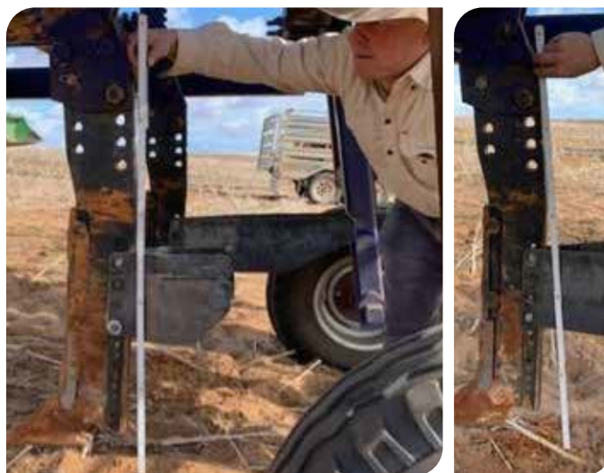
Figure 2. Deep ripper tine with short (250 mm) inclusion plates (left) and long (600 mm) inclusion plates (right).
