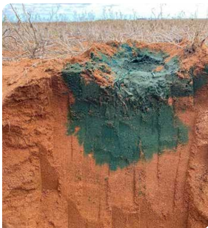
Figure 1. Soil pit dug in a constrained sandy soil type, blue dye was used to exemplify how water moves throughout the soil profile in relation to structure type, soil horizons and soil constraints.
