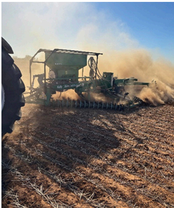
Figure 1. Kelly Engineering's – Kelly Chain sowing barley at Wandearah in 2025. Note barley is broadcast prior to the chain pass using an onboard hopper and air distribution system
